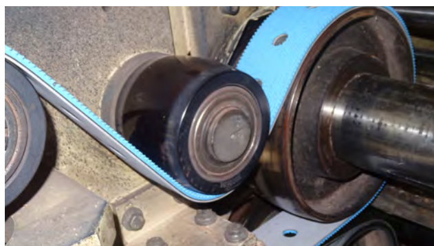
Polyamide foil tensile member offer high flexibility and edge stability.
